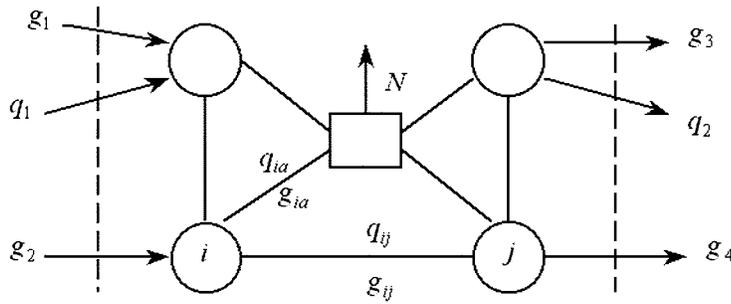
Figure 1. Open thermodynamic system with transformer.
