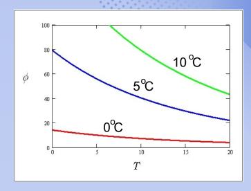
Dependency of the air humidity with respect to indoor temperature T is shown in the picture for three different values of outdoor temperature.
