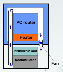
The box has two sections: the first, insulated, contains the network equipment; in the second, uninsulated, the accumulator and the power supply unit are placed. With this design, Thermobox needs neither heater nor fan when the outdoor temperature is between –10 and +25 degrees Celsius, which is typical for central Russia.
