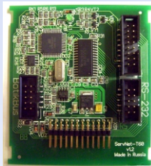
ServNet-T60: blade control card, 80×70 mm
