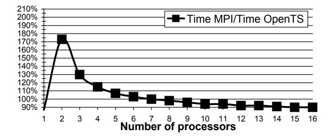
Performance comparison has been done with the "chess board scene" (scenes/advanced/chess2.pov taken from original POV-Ray distribution) with the scene width and height set to 1500. The chess board scene has 430 primitives in objects and 41 in bounding shapes. The graph, displaying the ratio between execution times MPI POV-Ray 3.50c and Open TS is presented above.
